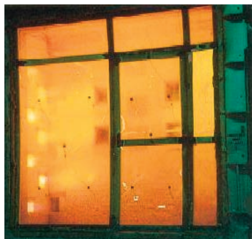
Glazed steel door and screen under fire test
