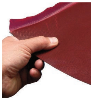
Intumescent material in sheet form
