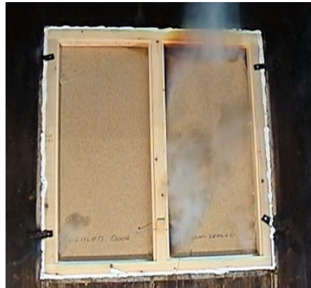
Without smoke seals, smoke passes around fire doors in the early stages of a fire - see unsealed right hand door
